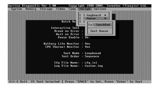
Select 'Test Mouse' or press **F8** to run the test. The prompt information would be displayed in the screen as below. This test item needs user to verify whether the mouse works normally.
