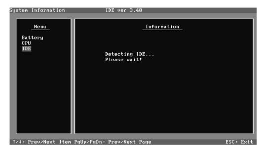
On the left column of the above screen, the detected hardware components are listed. The corresponding information of the detected hardware components is displayed on the right of the screen. It displays the current running status information of the check program. The name of the program is marked on the top of the screen. At the bottom, the function keys are listed for user operation. During the detection, keyboard operation is invalid.
