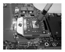
Figure 4-16 Applying silicon grease
